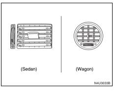
Use the lever located in the center of each outlet to change the direction of the airflow. Use the thumbwheel located next to the outlets to turn them on and off.
